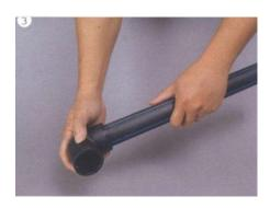
Quickly remove the heater and pressurize the two ends to be joined. After it is completed, check the appearance.
