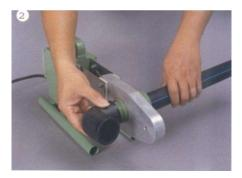
Connect the pipe with the fitting and insert into the welding head. Apply pressure to reach a certain depth (as shown in the table below)
