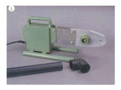
Install the welding head on the welding machine and heat it up to  $220^{\circ}\mathrm{C}$
